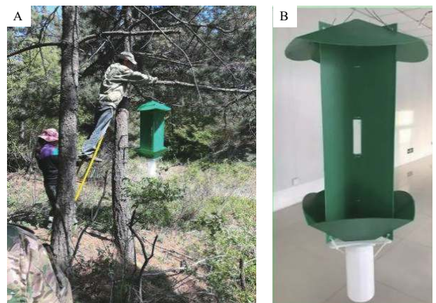
(A. 悬挂诱捕器; B. ZM-80B型诱捕器, APF-I型诱芯) (A. Hanging trap; B. ZM-80B trap, APF-I attractant)
